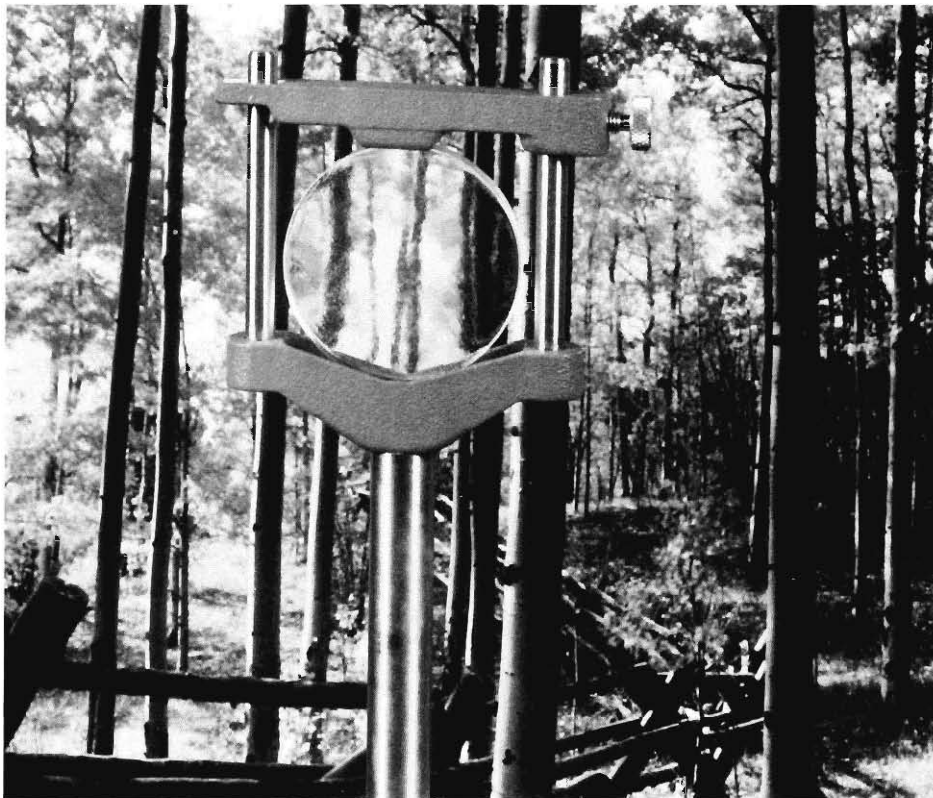
Fig. 4. Is this optical element useful? The distorted sodium chloride window in this picture was used as an aberrator in the experiment of Fig. 3 to illustrate the healing properties of phase-conjugate reflection. This technique becomes an attractive option when the quality of key optical components is limited by expense or technical considerations.
